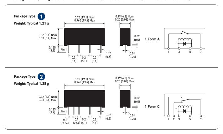
**Important:** Where the optional internal diode is fitted or for all Form B types, the correct coil polarity must be observed, as shown by the + symbol on the schematics.
