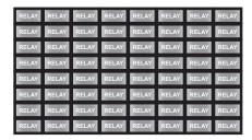
In this small area of only  $2.16 \times 1.2$  inches  $(5.48 \times 3.05 \text{ cm})$ , it is possible to construct an  $8 \times 8$  matrix - 64, 1 Form A relays.
