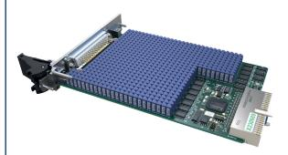
A total of 606 Series 124 relays on an example ultra-high-density PXI module illustrates the packing density of these extremely small Reed Relays.
