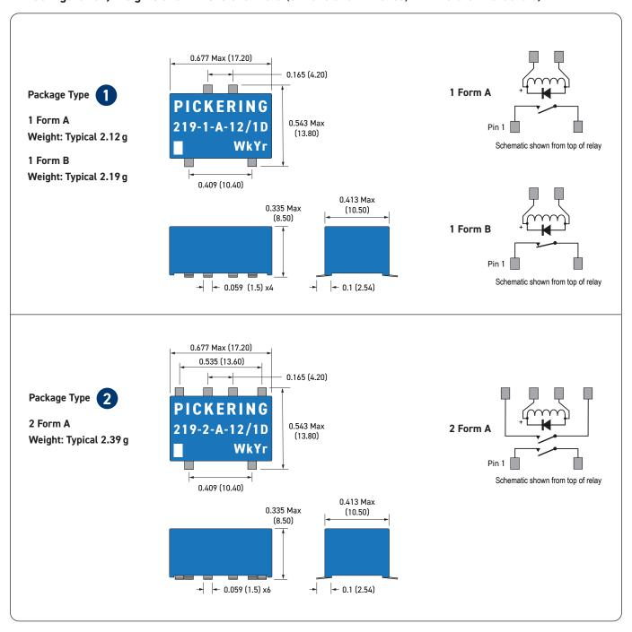
**Important:** Where the optional internal diode is fitted or for all Form B types, the correct coil polarity must be observed, as shown by the + symbol on the schematics.
