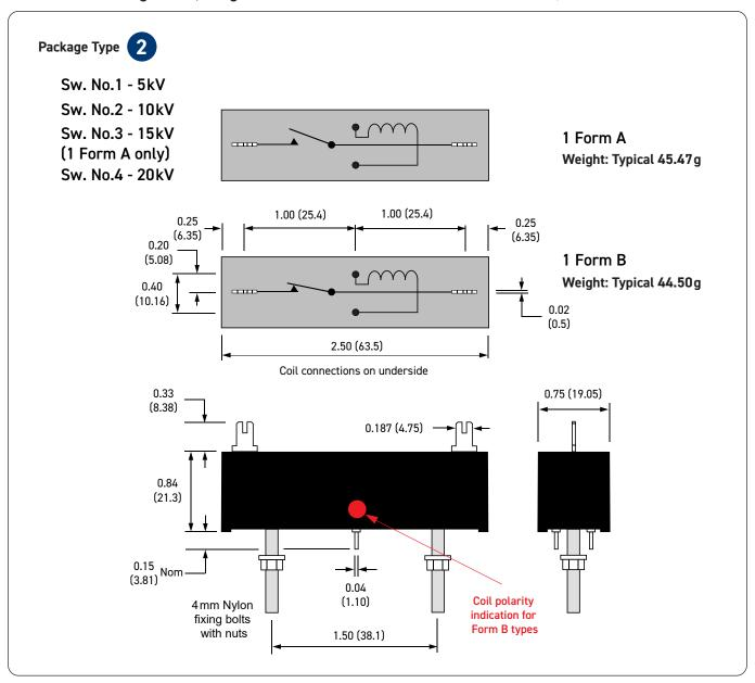
**Important:** For all Form B types, the correct coil polarity must be observed. The positive connection is shown by the red spot on the package.
