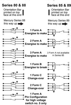
**Important:** Where the optional internal diode is fitted or for all Form B types, the correct coil polarity must be observed, as shown by the + symbol on the schematics.
