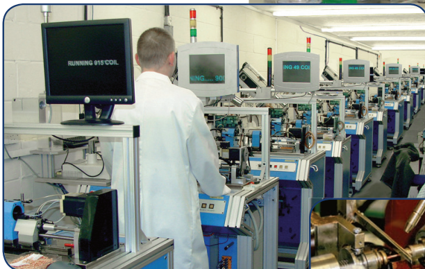
Formerless Coil Winding on fully automatic machinery
