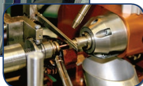
Formerless Coil Winding on fully automatic machinery
