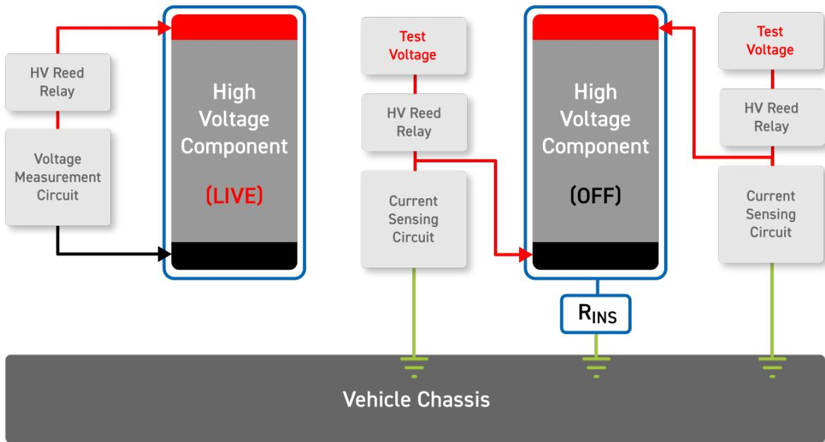
Figure 1 Voltage measurements (on the left) require connecting to a component (such as battery pack terminal) that could be at more than 400VDC. An insulation test (on the right) involves injecting a high voltage into a component and measuring the current that flows through a resistor of a known value (within the current sensing circuit) to the chassis. From that current, the insulation resistance ( $R_{INS}$ ) can be deduced.
