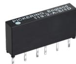
These devices have very low leakage currents (less than 1nA) and very high standoff voltages (a few kV) are achievable in small packaging. Switch contacts (the reeds) are hermetically sealed, so you don't get the same contamination/oxidation issues as with electromechanical relays.
