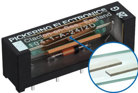
**Diagram 2** The maximum switching and minimum standoff voltages are high in a reed relay thanks to the gap between the reeds (shown in the inset) and the fact that they are in a vacuum. Insulation resistance is high thanks to pin spacing and the relay's base material. As for external shield clearance, this is not an issue when the EMI shielding is on the inside of the device.
