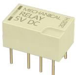
A popular and trusted technology but, because the contacts are not in a vacuum or inert gas, you need a large contact gap (and therefore relay body) to achieve a high standoff voltage.
