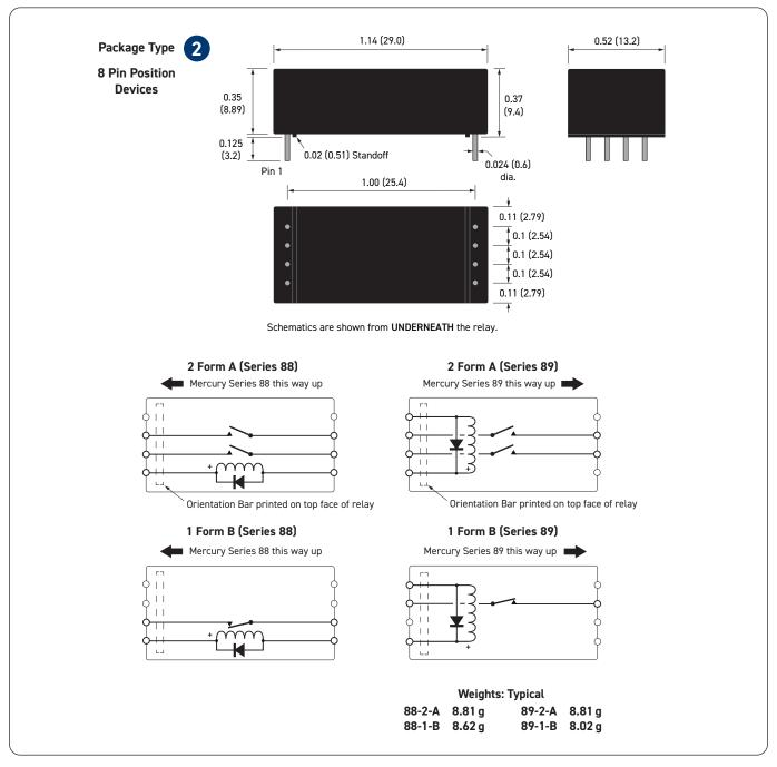
**Important:** Where the optional internal diode is fitted, the correct coil polarity must be observed as shown by the + symbol on the schematics.
