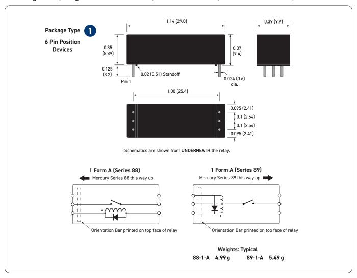
**Important:** Where the optional internal diode is fitted, the correct coil polarity must be observed as shown by the + symbol on the schematics.
