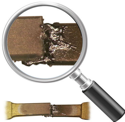
Bad contact weld due to switching very high current
